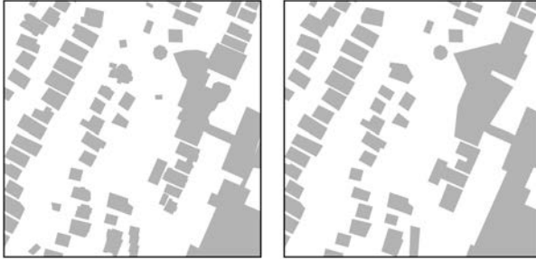
Figure 3.11. Map generalization showing a simplified layer after processes of selection, simplification, and aggregation—look closely!
